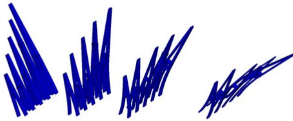
Fig. 2. Independently bending ribs forming pectoral fin curvature
