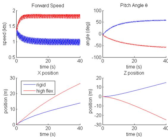
**Fig. 6. Simulated open-loop responses of vehicle to fin flapping with rigid ribs (blue) and fully flexible ribs (red).**
