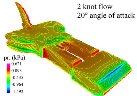
**Fig. 2. Test vehicle CFD drag analysis.**
