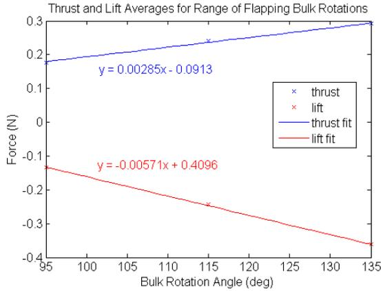
**Fig. 5. Thrust and lift forces produced over range of operating amplitudes.**
