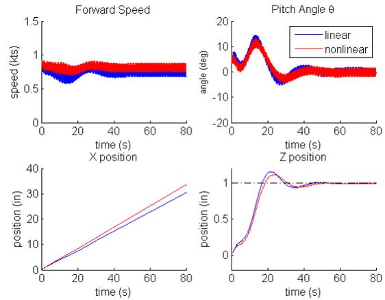
**Fig. 10. Simulated vehicle response of linear (red) and nonlinear (blue) systems to one meter depth change command.**
