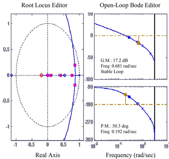
**Fig. 9. Stability analysis of discrete linear vehicle system using root locus and bode plots**
