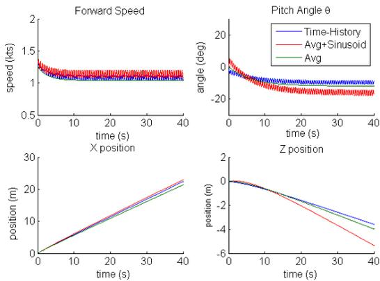
**Fig. 8. Simulated open-loop responses to fin flapping with fully described force time-histories (blue), average force values plus sinusoidal variation (red), and average force values (green).**
