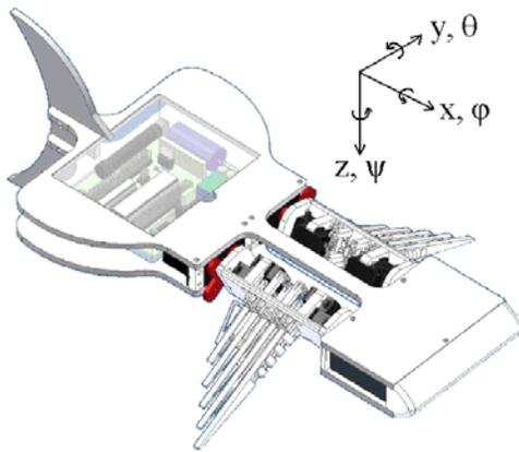
**Fig. 1. Test vehicle showing fins, electronics and fixed vertical and horizontal tails.**
