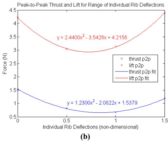
**Fig. 7. Individual rib deflection effect on thrust and lift generation (a) average force curves (b) peak to peak force amplitude curves.**
