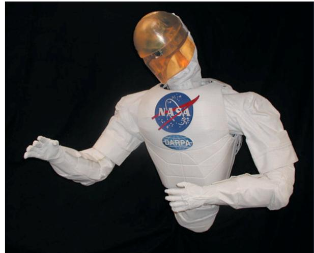
*Figure 5: Robonaut at NASA Johnson Space Center is a teleoperated robot with the full range of motion of the human upper body. It is directly teleoperated by a human operator who can see through Robonaut's "eyes" and affect hand and arm position with instrumented gloves.*
