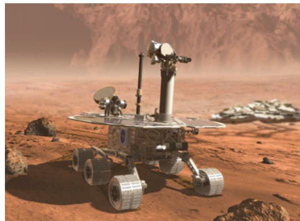
*Figure 3: Mars Exploration Rover illustrated departing its lander. MERs can navigate and avoid obstacles as may utilize this capability during their 2004 missions.*
