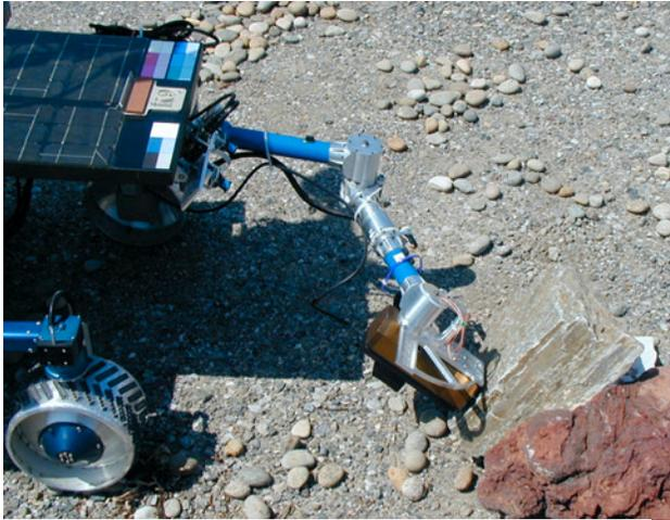
*Figure 6: NASA's K9 rover can approach a designated location then automatically determine the best measurement site, deploy its instrument to a rock, and collect science data in a single command cycle.*
