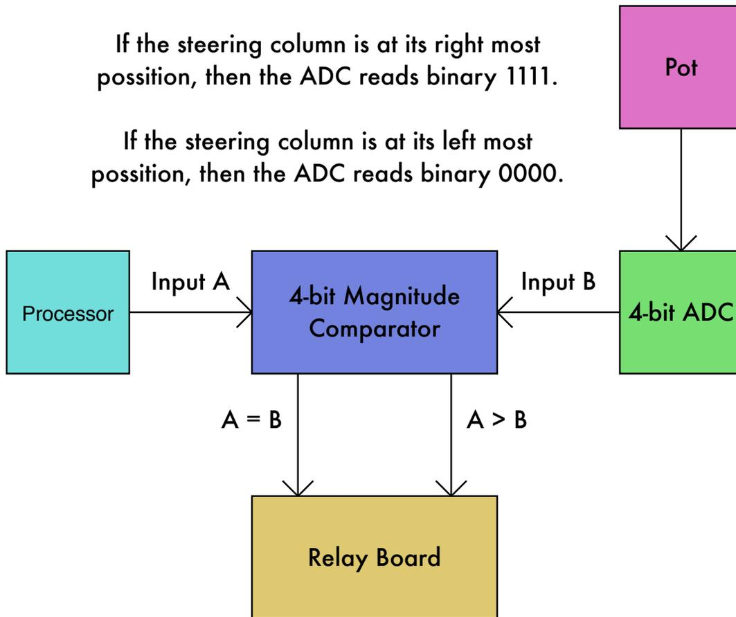
If  $A = B$  is high, then the power to the steering motor is switched off.
