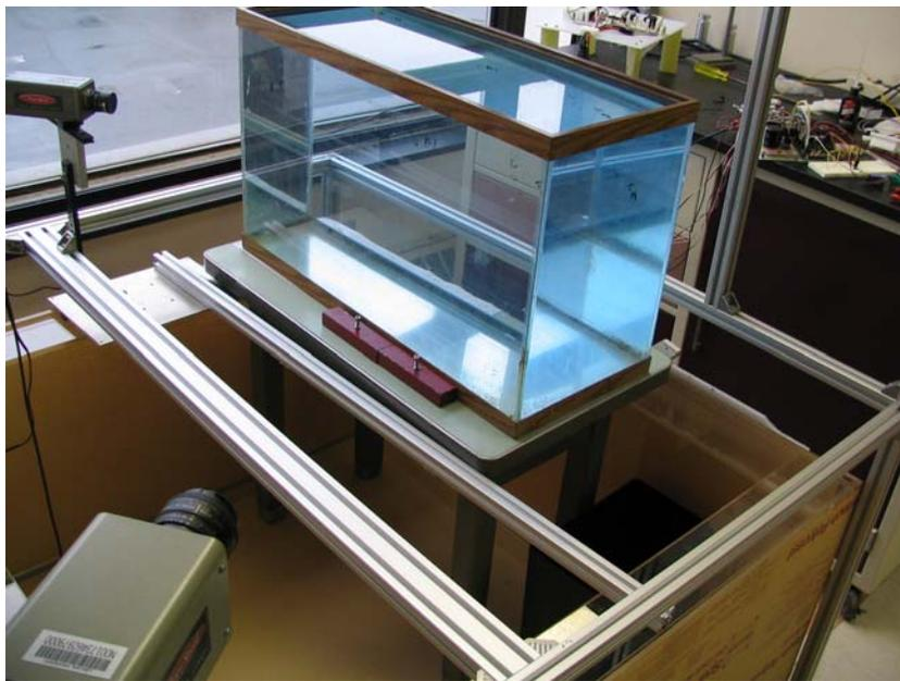
Fig. 8. Camera Slide System
